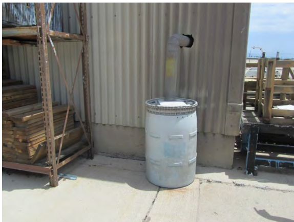
Photograph 29. Drum to capture sand blasting debris outside the west wall of the Velocity Air south hangar. View to the east.
