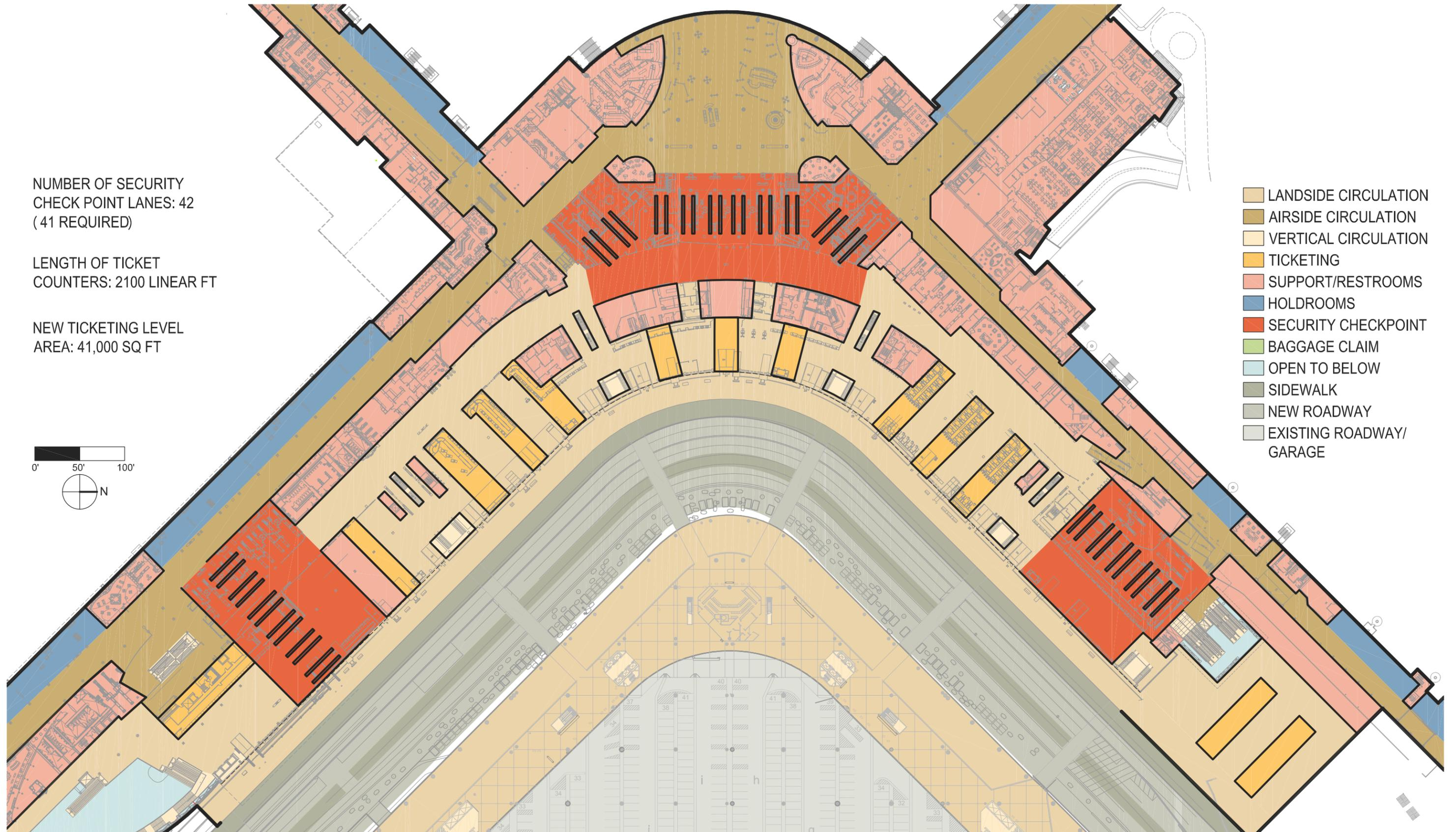
SEA MASTERPLAN - OPTION 1B - CONCOURSE LEVEL - EXPANDED FRONT FACADE / EXPANDED UPPER LEVEL ROADWAY
