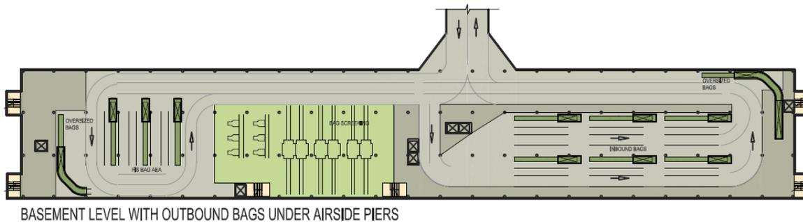
Figure 5 Architect suggested layout, basement level BHS at North Terminal
