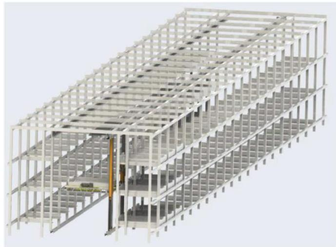
*Figure 12 Example of modular EBS storage system (source Beumer Group)*
