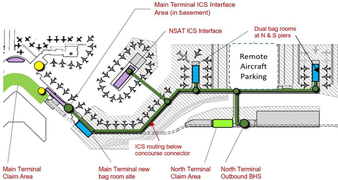
Figure 21 Possible Inter-Terminal connectivity of BHS facilities by ICS delivery/sortation system
