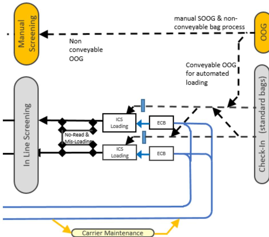
Figure 8 - Preferred EDS schematic diagram
