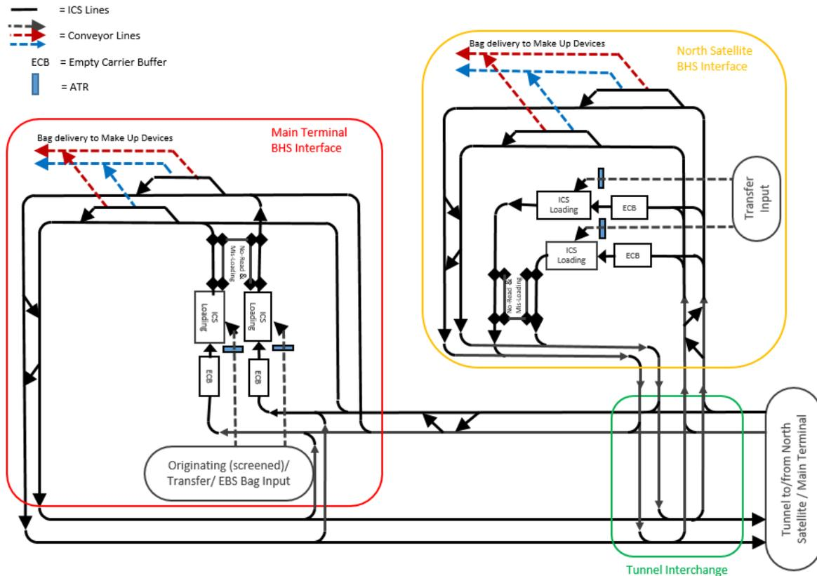
Figure 22 Overview of ICS delivery/sortation connectivity, North Terminal to other terminal areas
