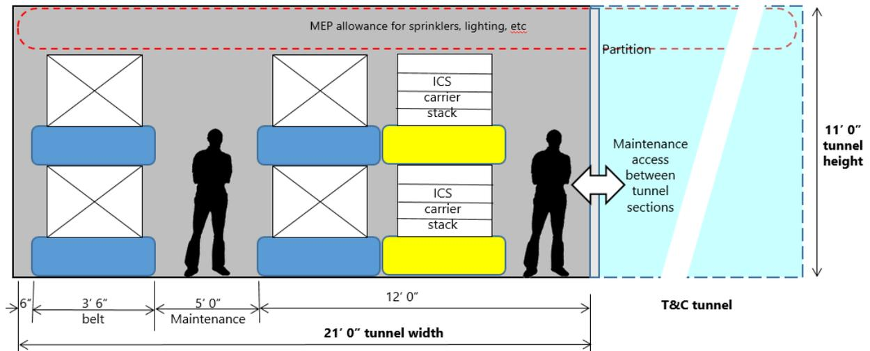
Figure 17 Modified tunnel configuration with ECB storage in tunnel
