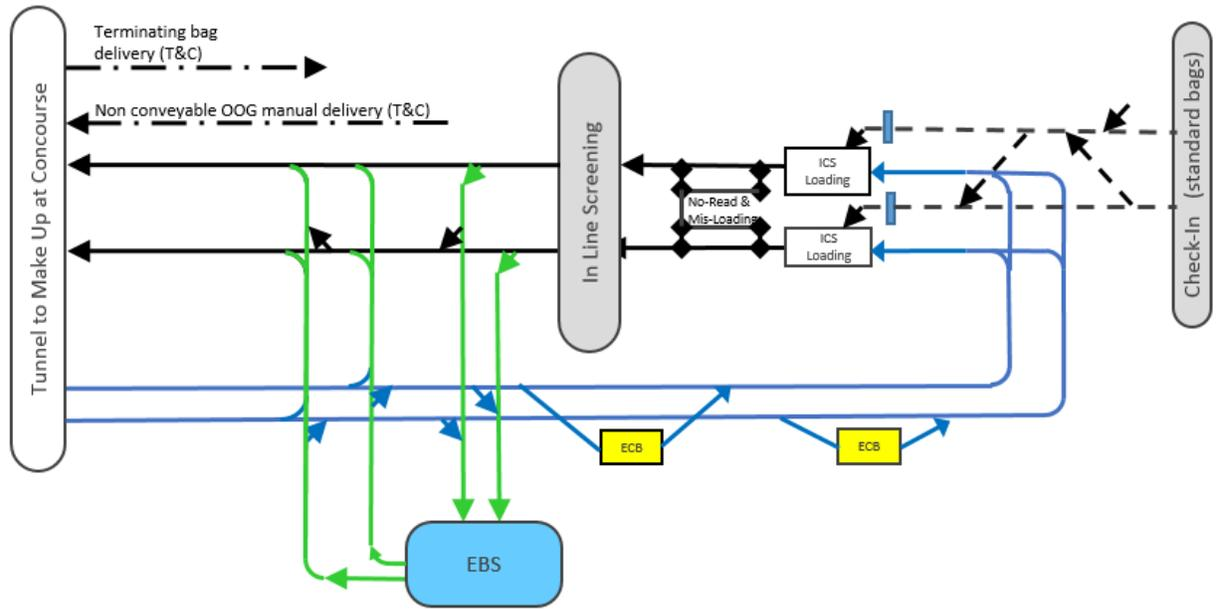
Figure 16 Modified MFD providing ECB storage in tunnel
