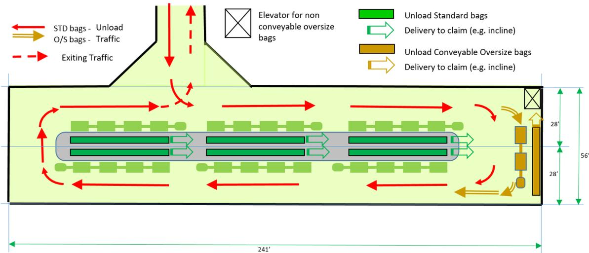
Figure 7 North Terminal Inbound Baggage Unload Area
