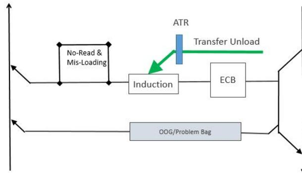
Figure 20 Transfer input and OOG problem bag area
