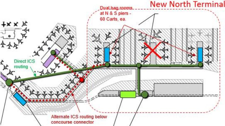
Figure 2 Alternate ICS routing to connect terminal areas
