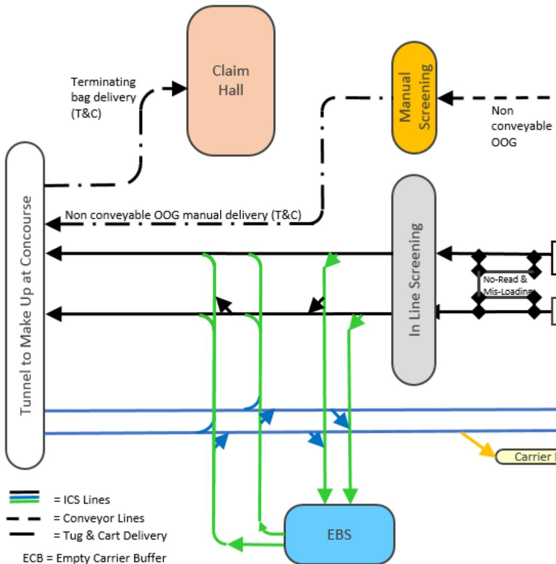
Figure 13 ICS and T&C delivery between N terminal processor and concourses
