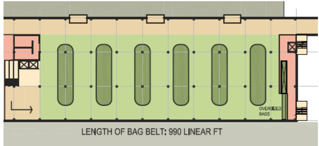
Figure 1 Proposed domestic claim layout, North Terminal
