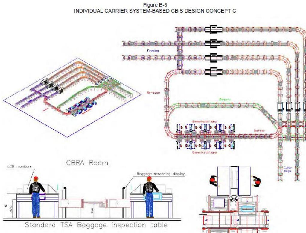
Figure 11 ICS based CBIS/CBRA concept example from PGDS-v5
