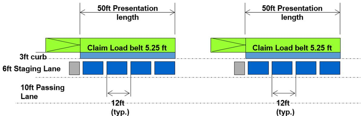
Figure 6 Possible layout approach for claim load belts
