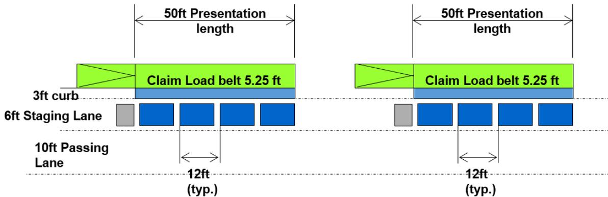
Figure 6 Possible layout approach for claim load belts. The spacing between adjacent claim load belts will vary depending on routing of delivery belts downstream of the incline section, but in any event it will need to provide clear headroom for load personnel below the incline and subsequent conveyors working at the adjacent claim load belt.
