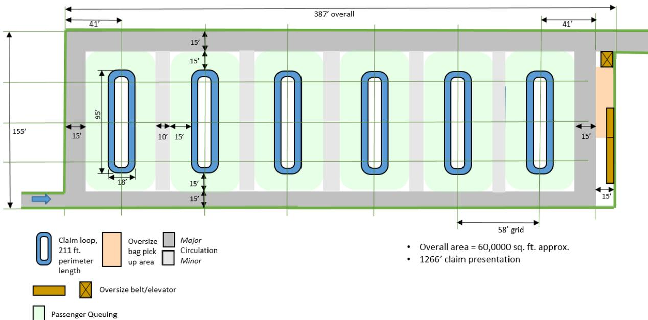
Figure 4 BHS Facility Space Requirements – Possible layout approach for claim hall
