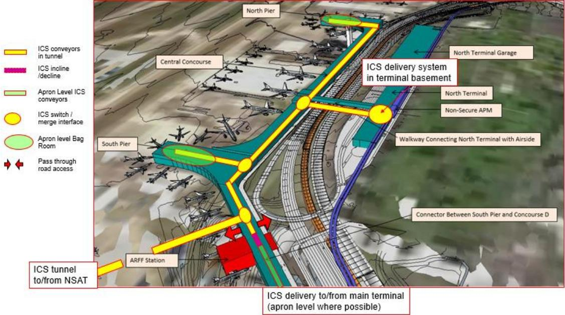
Figure 3 View illustrating ICS connectivity at North Terminal
