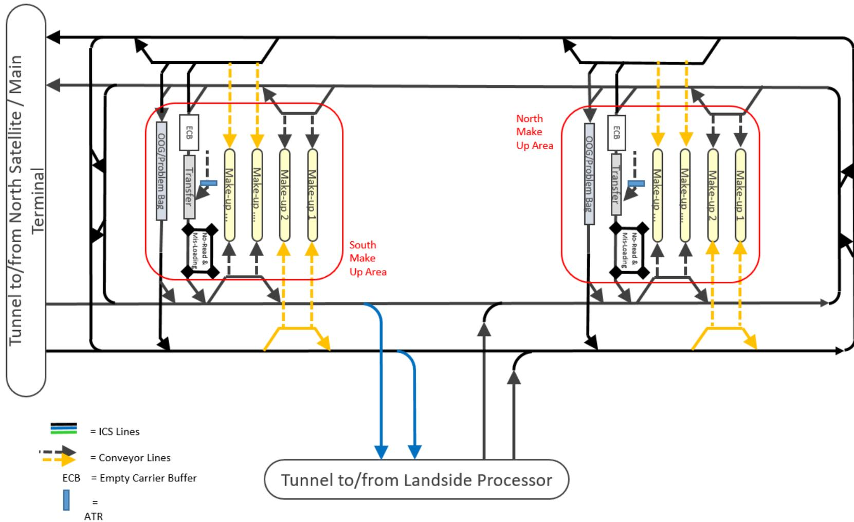
Appendix H - Main Terminal & North Satellite Interfaces - Material Flow Diagram
