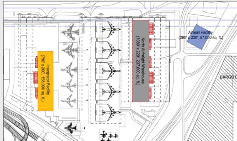
**Objective:** Determine how much of the forecast PAL 4 (2034) cargo requirements could be accommodated if the integrator (i.e., FedEx) warehouse remains in its existing location.
