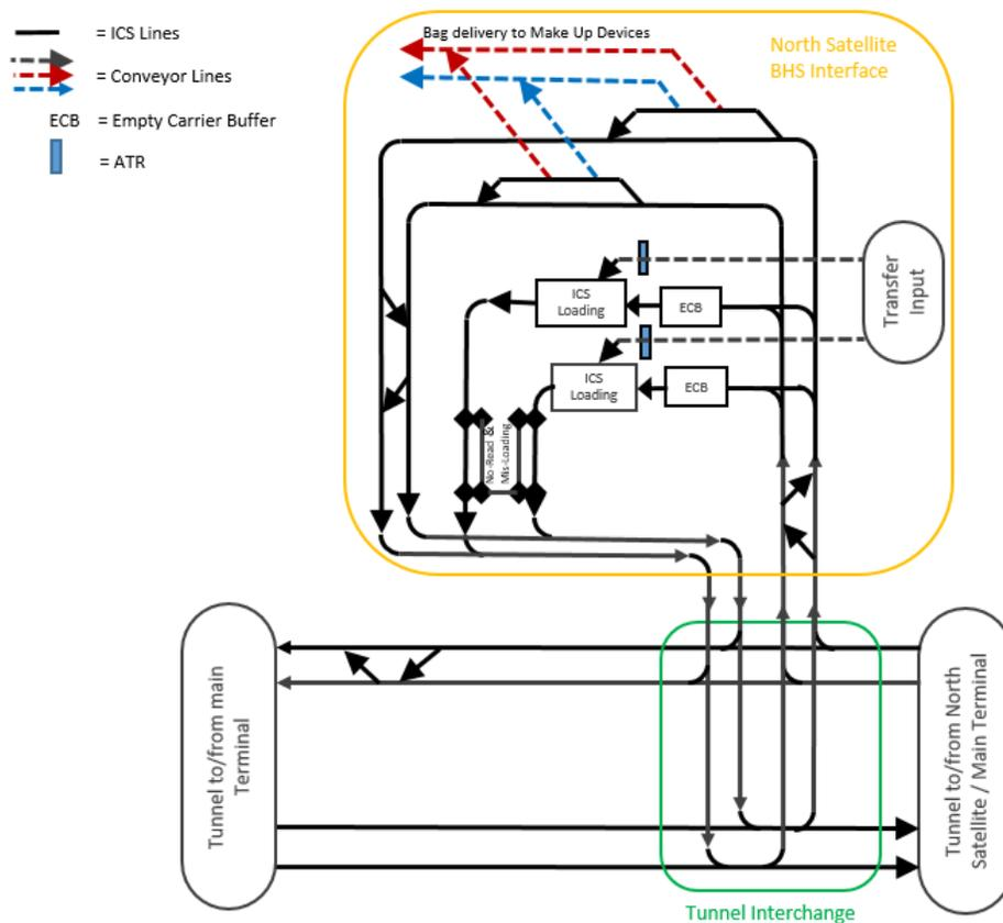
Figure 25 ICS connectivity North Terminal to North Satellite bag room
