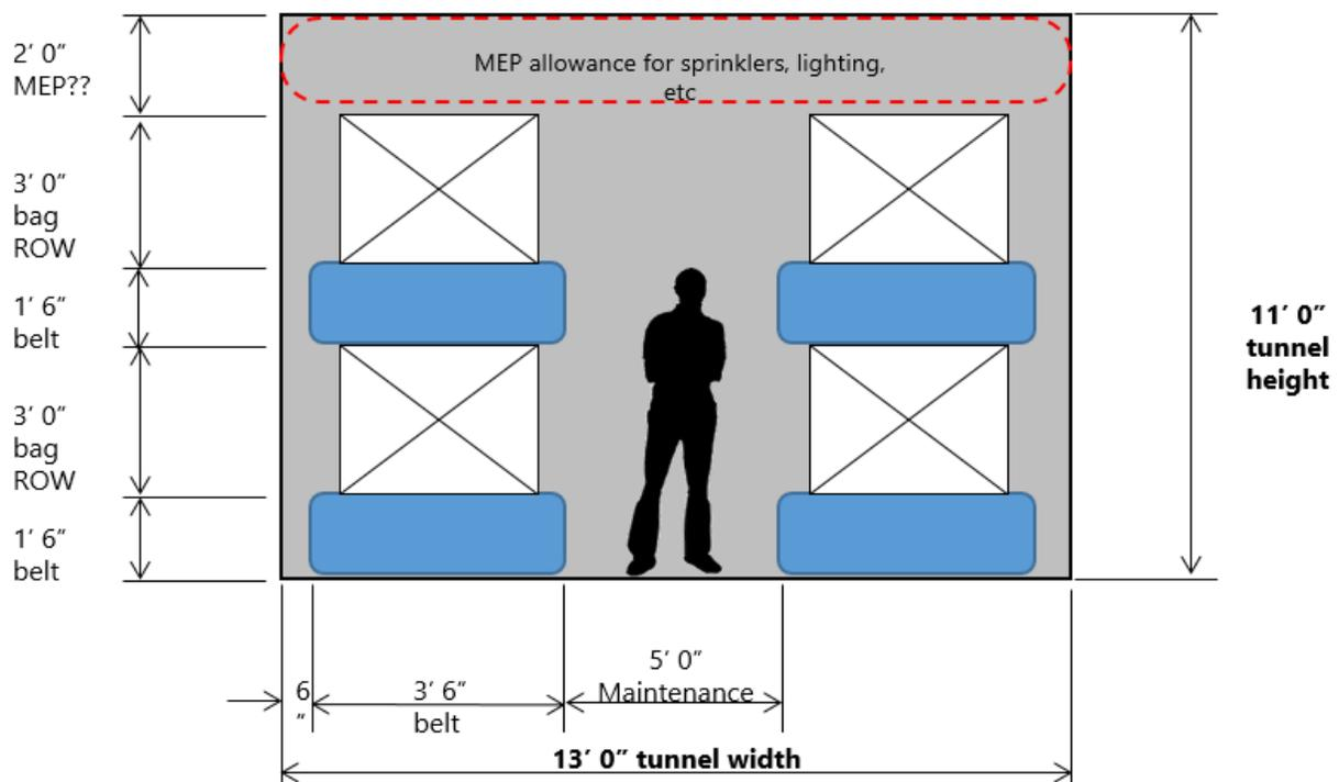
Figure 14 Possible Tunnel Configuration (4 lines)
