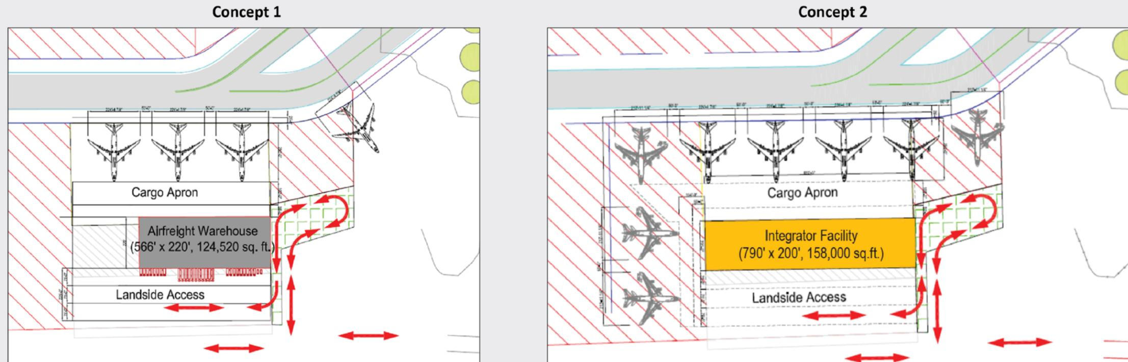
**Objective:** Provide airfreight warehouse capacity and freighter parking positions to supplement the facilities provided in the north cargo area.
